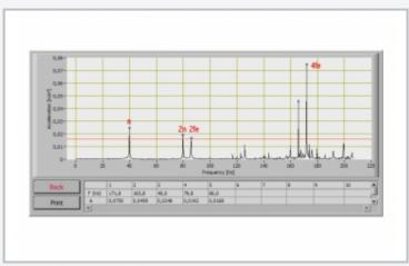
Typical spectrum of an electric motor rotary frequent vibration with n, 2n because of balance error power frequent vibration with 2fe, 4fe because of magnetic forces
