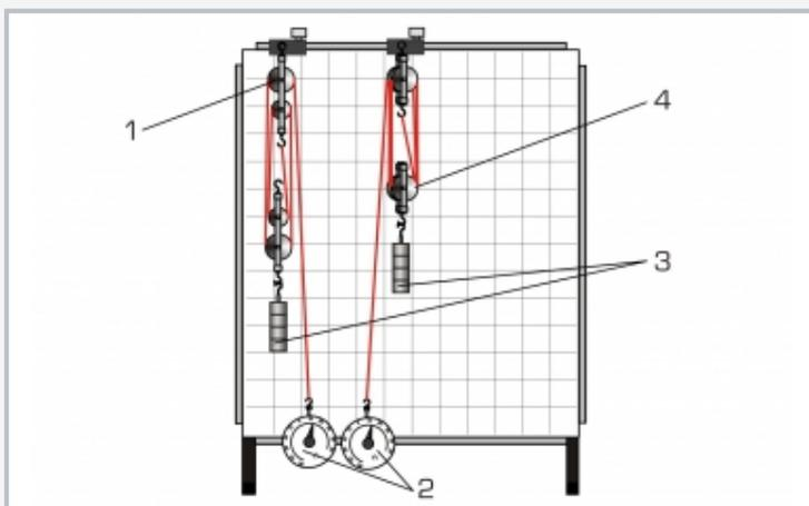
Experimental setup with the pulley blocks supplementary set (TM 110.02):
