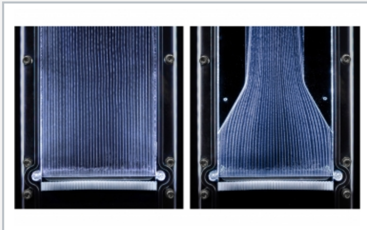
Visualisation of streamlines with hydrogen bubbles left: flow channel without change in cross-section, right: flow channel with inserted models for change in cross-section
