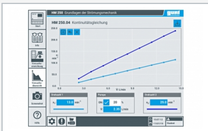
Intuitive user interface on the HM 250 touch screen: graphic display of the measured values, speeds of the two impellers in different cross-sectional flow areas of the pipe section
