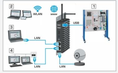
Connection of the Web Access Box shown by the example of ET 400 1 USB connection with selected GUNT device (here: ET 400), 2 connection of end devices via WLAN, 3 direct LAN connection of an end device, 4 connection of end devices by integrating the Web Access Box into the customer's own network
