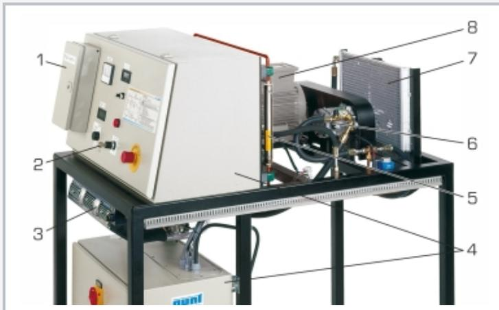
1 box with fault buttons, 2 ignition key, 3 air cooler with three-stage fan, 4 switch cabinet, 5 flow meter, 6 compressor, 7 condenser with fan, 8 electric motor
