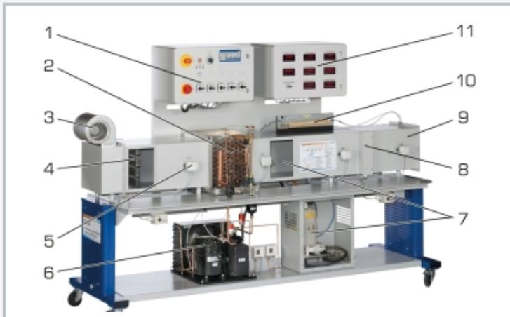
1 controls, 2 air cooler (direct evaporator), 3 fan, 4 air preheater, 5 temperature sensor, 6 condensing unit, 7 air humidifier, 8 air reheater, 9 air duct, 10 inclined tube manometer, 11 displays
