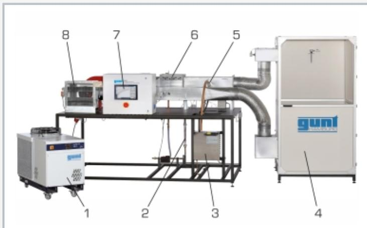
1 water chiller, 2 flow meter, 3 steam humidifier, 4 climatic chamber, 5 steam distributor (humidifier), 6 air cooler, 7 PLC, 8 outer air inlet with fan; covered: air heater
