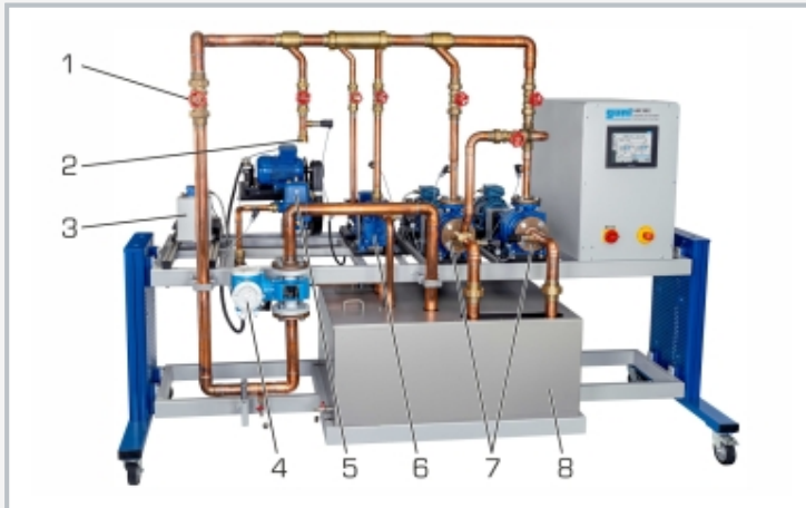
1 flow control valve [at outlet], 2 connection for additional pump, 3 motor for additional pump, 4 flow rate sensor, 5 piston pump, 6 side-channel pump, 7 centrifugal pump, 8 storage tank
