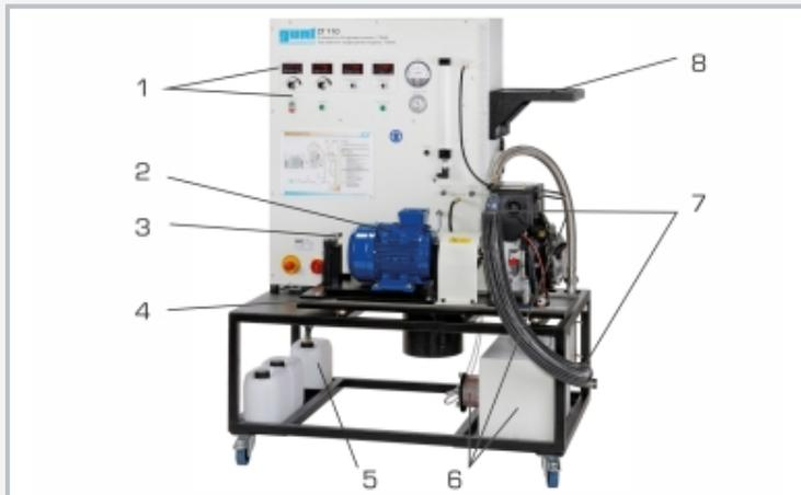
1 display and control panel, 2 asynchronous motor, 3 force sensor (torque), 4 base plate, 5 fuel tank with pump, 6 stabilisation tank with air filter and air hose, 7 exhaust gas connection, 8 shelf, e.g. for CT 100.13
