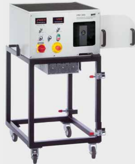
HM 365 Universal drive and brake unit
