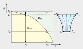
Pressure and velocity distribution along the streamlines: the yellow area represents the range of static pressure, whereas the green area represents that of the dynamic pressure; the sum of the two pressures gives the total pressure **p**0
