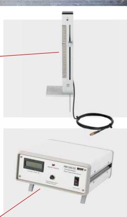
The water level in the open channel is measured with the electronic level gauge. The level gauge can be attached at any point on the side wall of the duct. The water level is determined by means of a sliding probe. The position of the probe can either be read directly from the scale on the level gauge or displayed digitally on the main unit.
