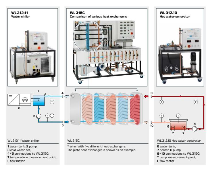
The accessories WL 312.11 Water chiller and WL 312.10 Hot water generator supply cold and hot water for the experiments independent of the laboratory supply. This means that the trainer can be operated as a stand-alone system with a closed water circuit.
