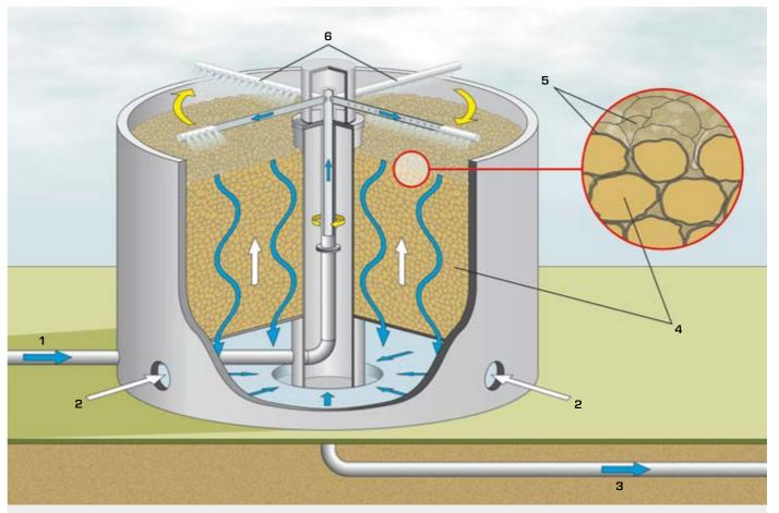
How a trickling filter works:
