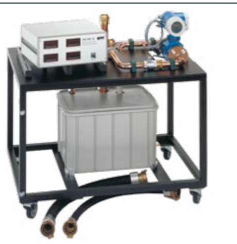
HM 365.10 Supply unit for water pumps
